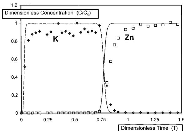
FIGURE 1. Biosorption column breakthrough profiles. Experimental data and IMPACT model simulations for *K-Sargassum* biosorbent. Feed solution pH 4.5; [Zn] = 3 mequiv/L; feed rate: 8 cm<sup>3</sup> min<sup>-1</sup>. K outlet concentration (◆) experimental points; (---) IMPACT simulation. Zn outlet concentration (■) experimental points; (—) IMPACT simulation.
