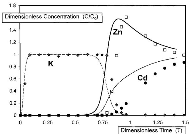
FIGURE 2. Biosorption column breakthrough profiles. Experimental data and IMPACT model simulations for *K-Sargassum* biosorbent. Feed solution pH 4.5; [Zn] = [Cd] = 1.5 mequiv/L; feed rate: 8 cm<sup>3</sup> min<sup>-1</sup>. K outlet concentration (◆) experimental points; (---) IMPACT simulation. Zn outlet concentration (■) experimental points; (—) IMPACT simulation. Cd outlet concentration (●) experimental points; (— · —) IMPACT simulation. (IMPACT calculations ceased at  $T = 1.4$ ).
