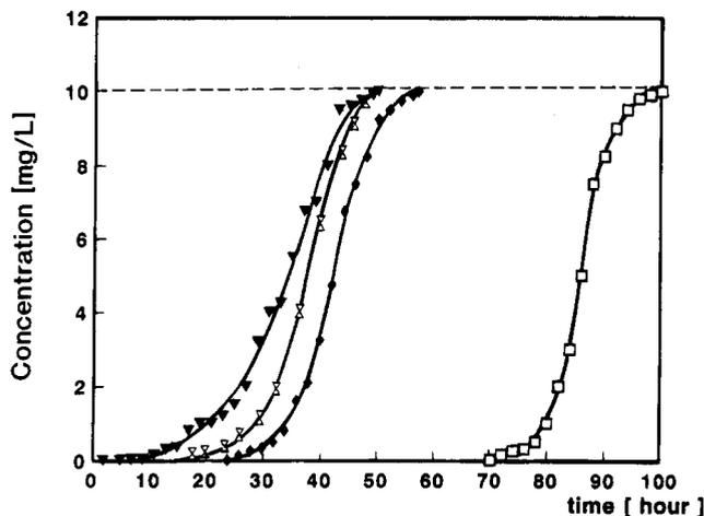
**Figure 6.** Continuous-flow fixed-bed column sorption of cadmium with reinforced *Ascophyllum nodosum* biosorbent (FCAN). Profiles of breakthrough curves for different sorption column feed flow rates (loadings): (□)  $2.4 \text{ L h}^{-1} \text{ cm}^{-2}$ ; (◆)  $4.8 \text{ L h}^{-1} \text{ cm}^{-2}$ ; (⊗)  $7.2 \text{ L h}^{-1} \text{ cm}^{-2}$ ; (▼)  $9.6 \text{ L h}^{-1} \text{ cm}^{-2}$  (Volesky and Prasetyo, 1994).
