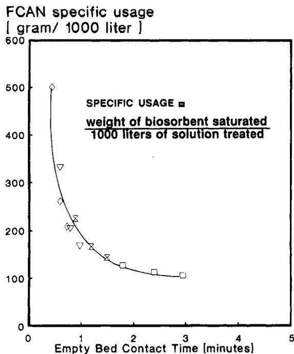
**Figure 7.** Effect of the sorption column liquid residence time on the specific usage of biosorbent FCAN derived from brown seaweed *Ascophyllum nodosum*. Flow rate: (□)  $2.4 \text{ L h}^{-1} \text{ cm}^{-2}$  and (◇)  $4.8 \text{ L h}^{-1} \text{ cm}^{-2}$  at loadings (◇)  $4.8 \text{ L h}^{-1} \text{ cm}^{-2}$  and (▽)  $4.8 \text{ L h}^{-1} \text{ cm}^{-2}$  (Volesky and Prasetyo, 1994).
